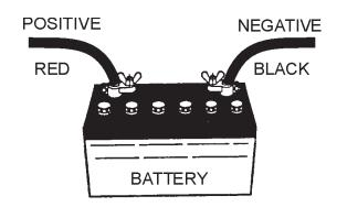
Figure 27. Battery Connections
